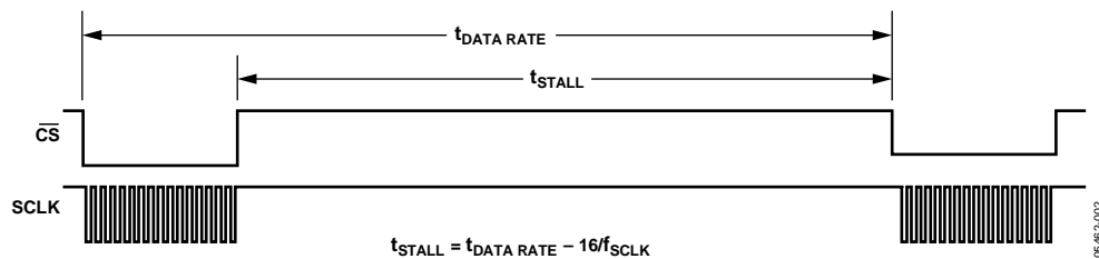
Figure 2. SPI Chip Select Timing
