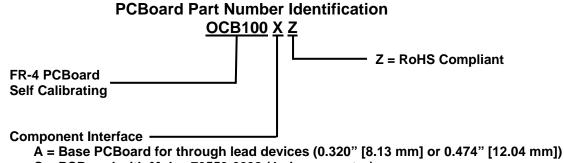
C = PCBoard with Molex 70553-0038 (4 pin connector)
