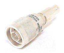
Microlab XA series diode mounts are general-purpose video detector mounts designed to accommodate commonly available diodes (e.g. point contact, Schottky, etc.). They are constructed in two detachable sections to allow access to the crystal. Both ends of the diode are held by beryllium copper contact springs to maintain uniform contact. Note that diode is not supplied.
