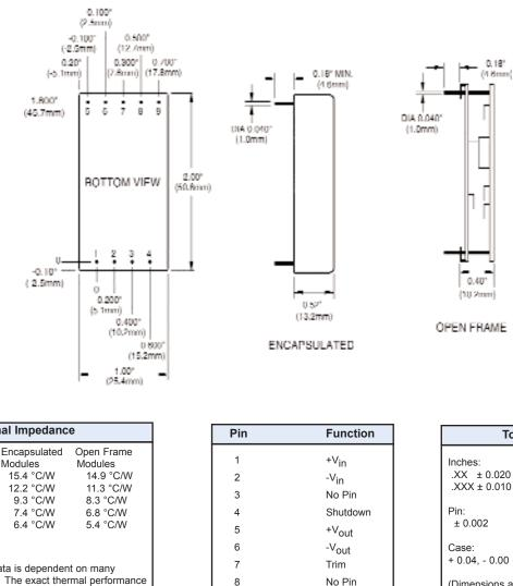
TolerancesInches:(Millimeters).XX  $\pm 0.020$ .X  $\pm 0.5$ .XXX  $\pm 0.010$ .XX  $\pm 0.25$ Pin: $\pm 0.002$  $\pm 0.002$  $\pm 0.05$ Case: $\pm 0.04$ , -0.00 $\pm 0.04$ , -0.00 $\pm 1.0$ , -0.00(Dimensions as listed unless otherwise specified.)
