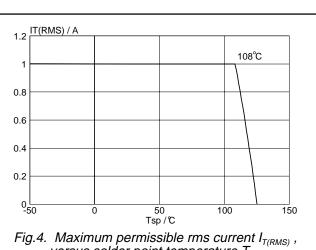
versus solder point temperature  $T_{sp}$ .
