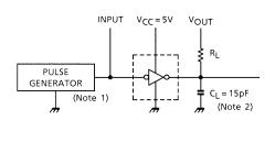
Note 1: Pulse Width 50  $\mu$ s, Duty Cycle 10% Output Impedance 50  $\Omega$ ,  $t_f \le 5$  ns,  $t_f \le 10$  ns
