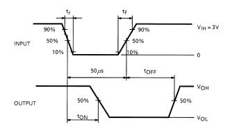
Note 1: Pulse Width 50  $\mu$ s, duty cycle 10% Output impedance 50  $\Omega$ ,  $t_f \le 10$  ns,  $t_f \le 5$  ns
