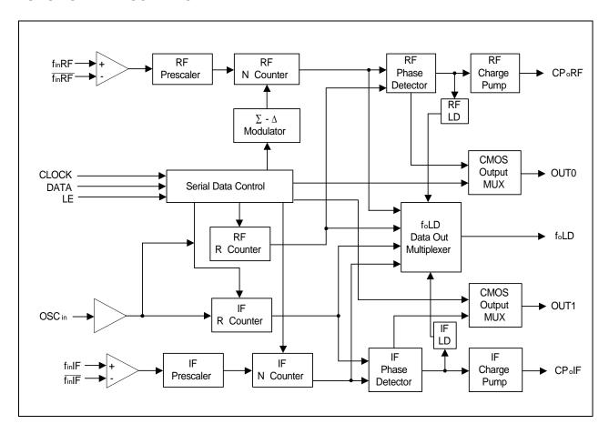
The Samsung S1M8836/37 is RF/IF dual frequency synthesizer IC which supports Fractional-N mode for RF PLL and Integer-N mode for IF PLL depending on a program control. S1M8836/37 combined with an external LPF and an external VCO forms PLL frequency synthesizer. The frequency synthesizer consists of prescalers, pulse-swallowed programmable N counters, programmable reference R counters, phase detectors, programmable charge pumps, analog LD(lock detector), serial data control, etc.
