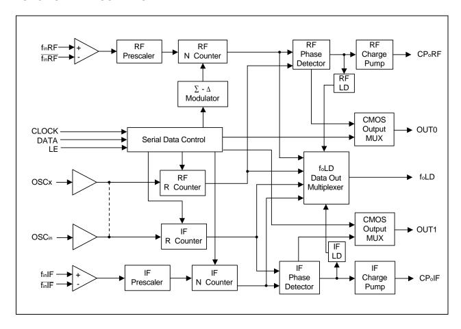
The Samsung S1M8831A/33 is RF/IF dual frequency synthesizer IC which supports Fractional-N mode for RF PLL and Integer-N mode for IF PLL depending on a program control. S1M8831A/33 combined with external LPFs and external VCOs forms PLL frequency synthesizer. The frequency synthesizer consists of prescalers, pulse-swallowed programmable N counters, programmable reference R counters, phase detectors, programmable charge pumps, analog LD (Lock Detector), serial data control, etc.
