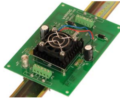
PAD112 INSTALLED IN EVALUATION KIT
