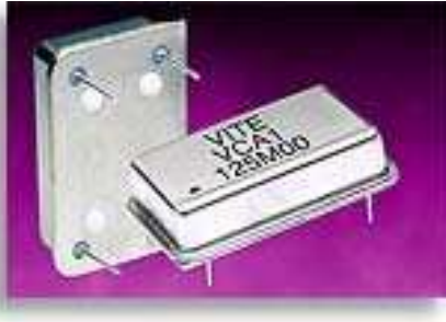
The VCA1 Crystal Oscillator
