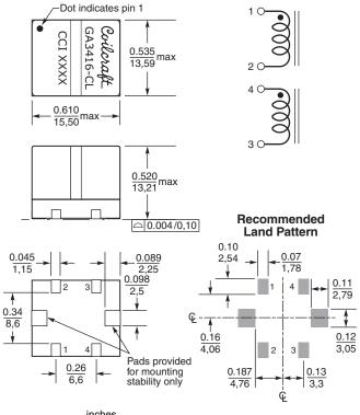
Dimensions are in  $\frac{\text{inches}}{\text{mm}}$
