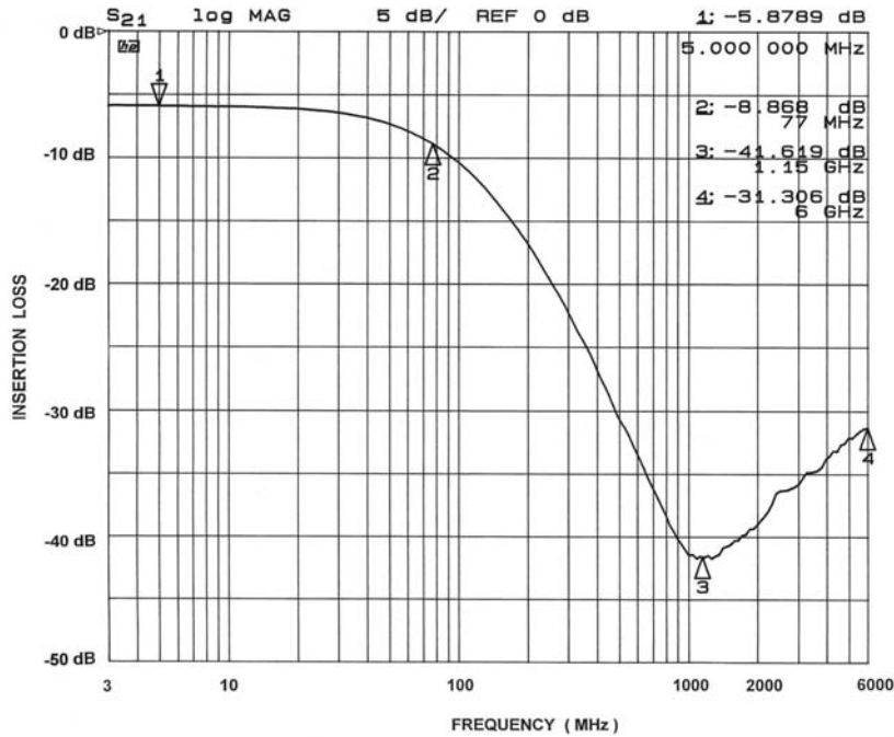
Figure 1. A1-C1 EMI Filter Performance
