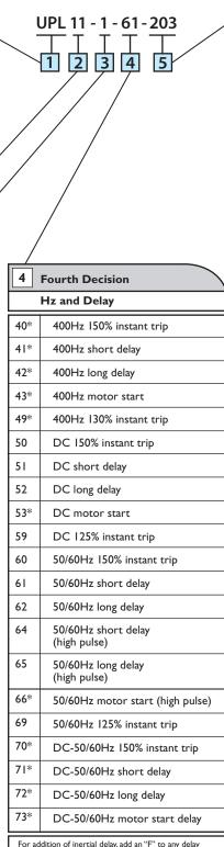
For addition of inertial delay, add an "F" to any delay number, except 40, 50, 60 and 70. \*Not available above 50 amperes.
