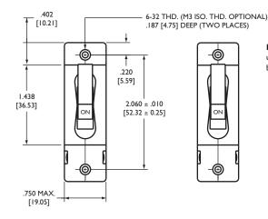
**Note:** Tolerance ± .015 [.38] unless noted. Dimensions in brackets [] are millimeters.
