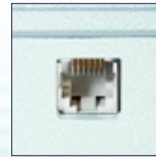
Integrated V.24 (RS232) interface with an RJ12 jack
