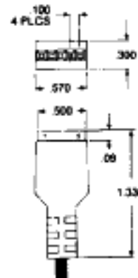
ALL SHIELDED CABLE VERSIONS COME WITH THE ABOVE CONNECTOR (MATING CONNECTOR PROVIDED)
