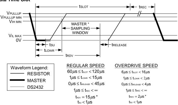
\*The optimal sampling point for the master is as close as possible to the end time of the  $t_{RDV}$  period without exceeding  $t_{RDV}$ . For the case of a Read-one time slot, this maximizes the amount of time for the pull-up resistor to recover the line to a high level. For a Read-zero time slot it ensures that a read will occur before the fastest 1-Wire device releases the line ( $t_{RELEASE} = 0$ ).
