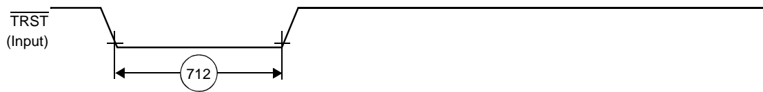
Figure 29. TRST Timing Diagram
