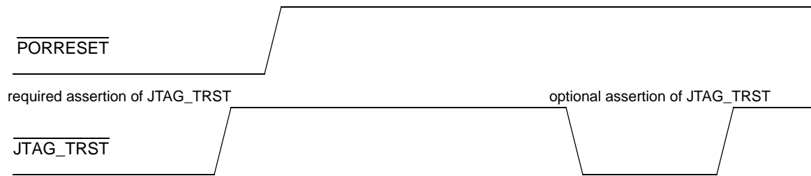
Figure 53. \overline{\text{PORRESET}} vs. \overline{\text{JTAG\_TRST}}
