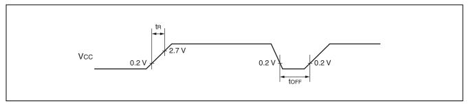
Note: If you change the power supply voltage too rapidly, a power on reset may occur. We recommend that you start up smoothly by restraining voltages when changing the power supply voltage during operation, as shown in the figure below. Perform while not using the PLL clock. However, if voltage drops are within 1 V/s, you can operate while using the PLL clock.
