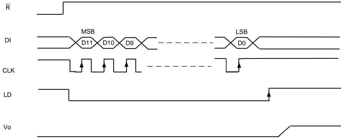
\*Input data is carried out LD signal low besides CLK signal positive edge. CLK, LD, is keep generally High level.
