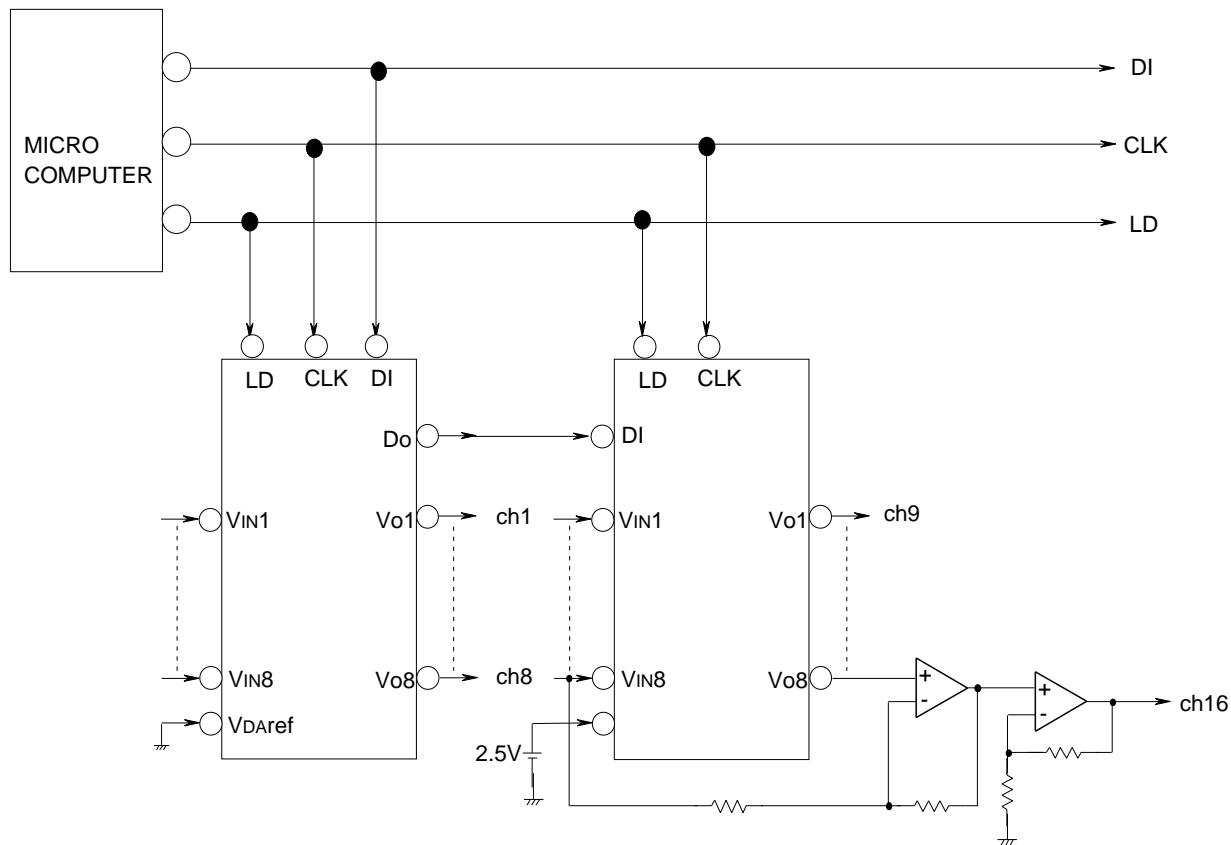
\*In this example,M62363X2 are connected in cascode.
