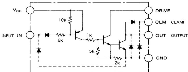
DRIVE, CLM,  $V_{CC}$ , and GND are common to channels 1 and 2.
