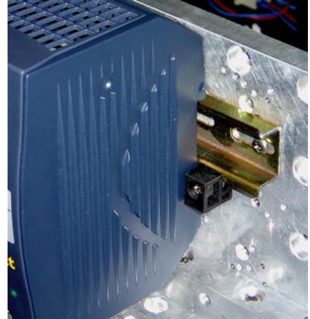
Fig. 23 One of 4 DIN-rail fixing brackets DMB-EWG.
