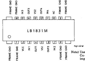
Note) Use one of the FRAME-GND pins for grounding. When the Cu-foild side is soldered, heat radiation can be more improved.
