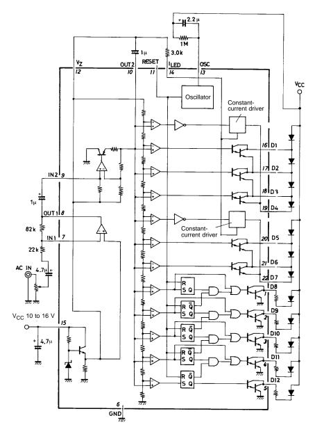
Unit (resistance:  $\Omega$ , capacitance: F)
