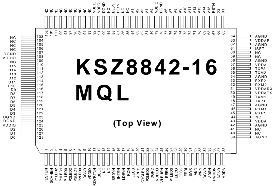
Figure 2. Standard – KSZ8842-16 MQL 128-Pin PQFP (Top View)
