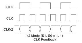
Using CLK as the feedback will always result in synchronized rising edges between ICLK and CLK. However, the CLK/2 could be a falling edge compared with ICLK. IDT recommends using CLK/2 feedback whenever possible. This will synchronize the rising edges of all three clocks.
