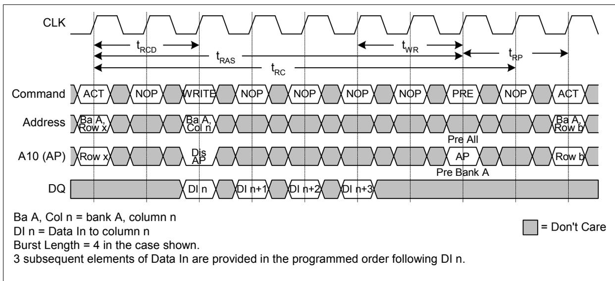
Figure 28 WRITE Burst (CAS Latency = 2)
