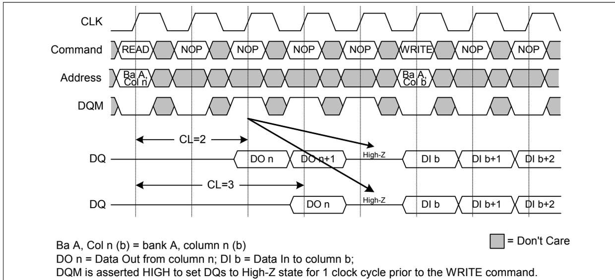
Figure 24 READ to WRITE Timing
