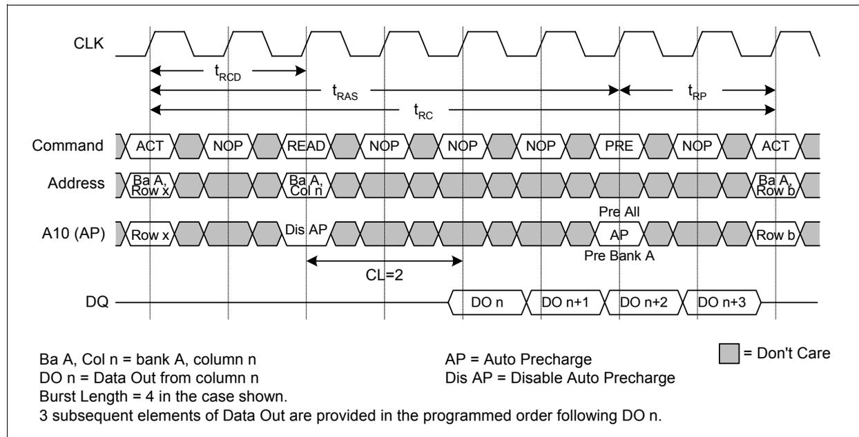
**Figure 16 Single READ Burst (CAS Latency = 2)**
