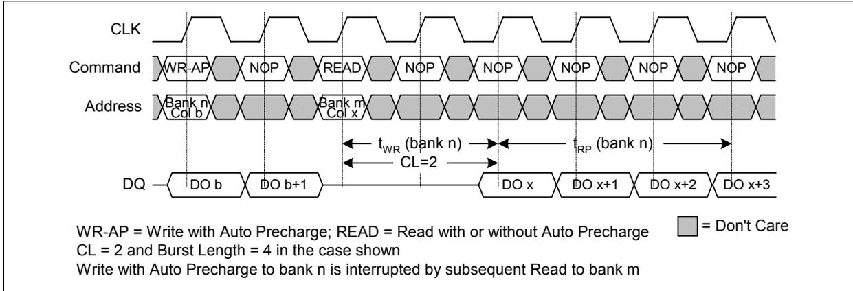
**Figure 42 WRITE with Auto Precharge Interrupted by READ**
