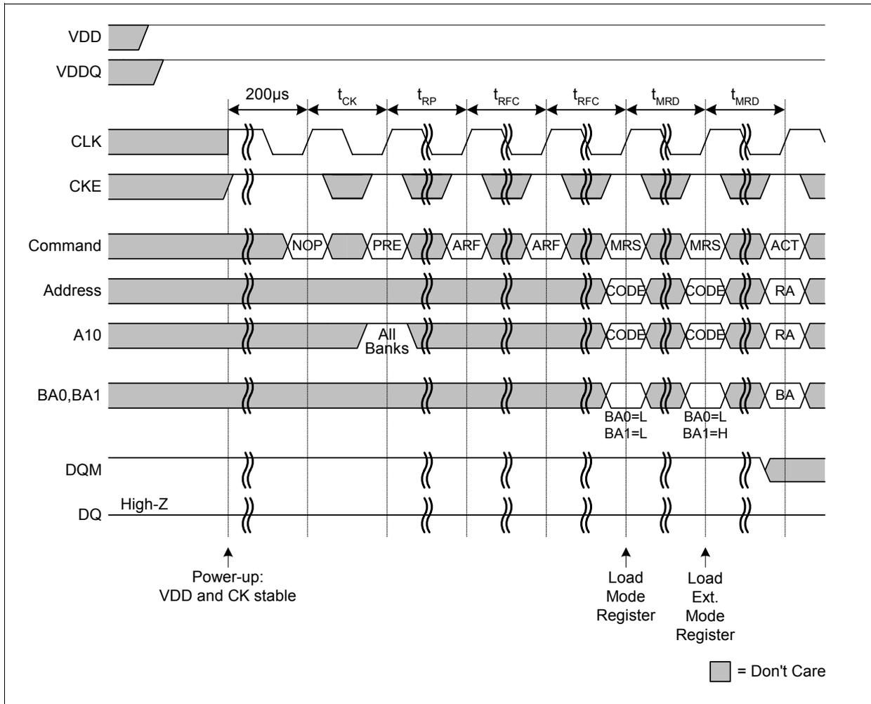
**Figure 4 Power-Up Sequence and Mode Register Sets**
