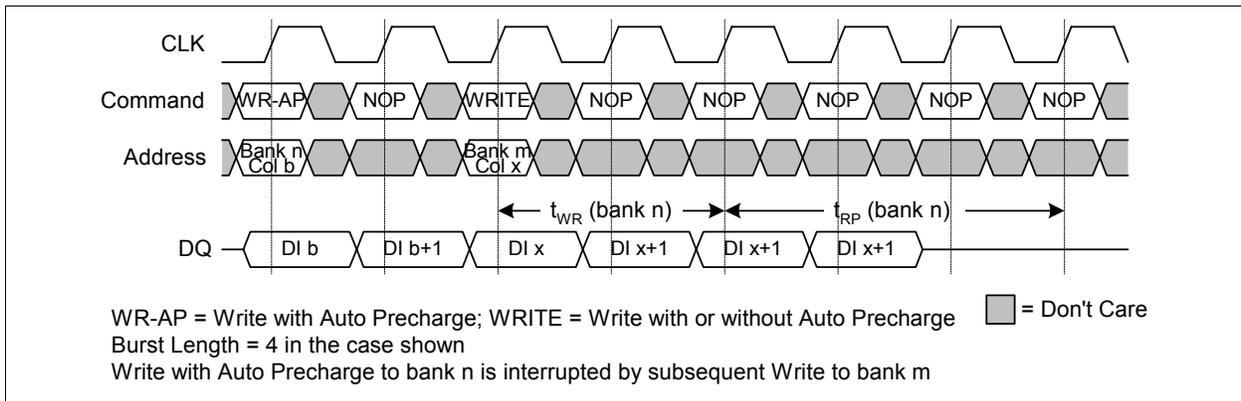
**Figure 43 WRITE with Auto Precharge Interrupted by WRITE**
