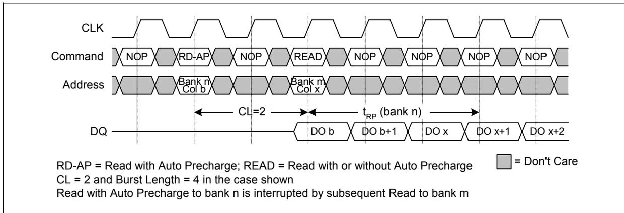
**Figure 40 READ with Auto Precharge Interrupted by READ**
