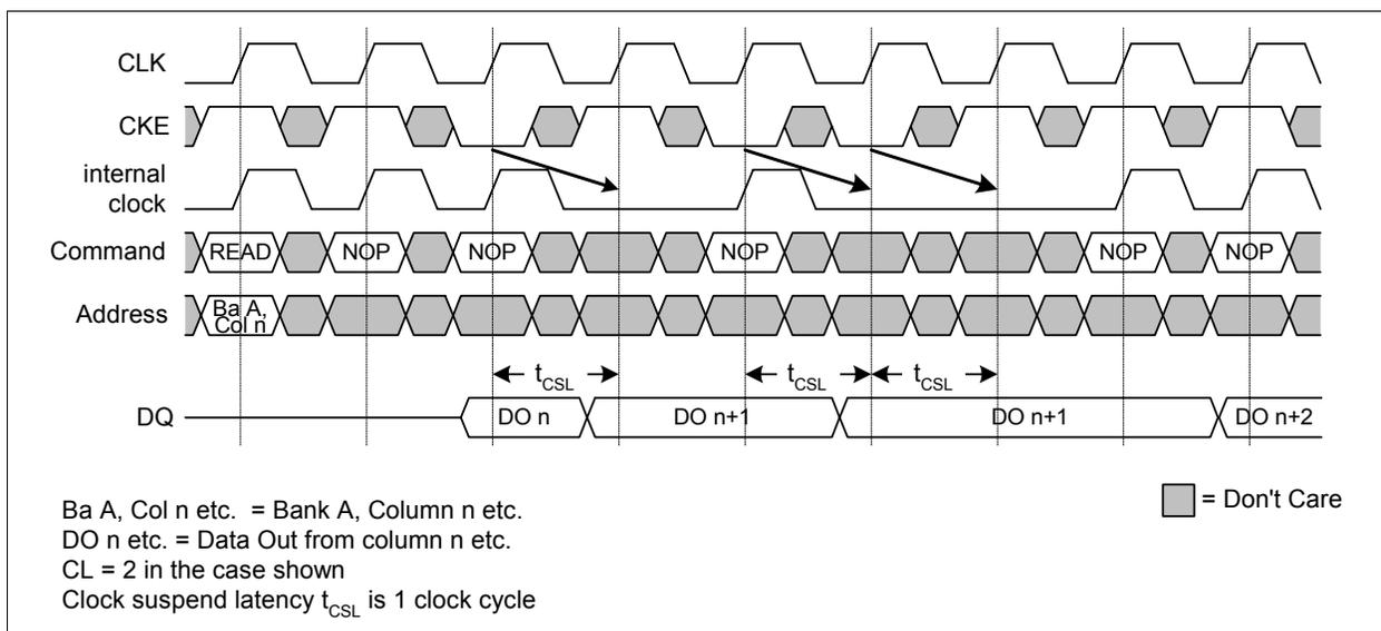
Figure 22 Clock Suspend Mode for READ Bursts
