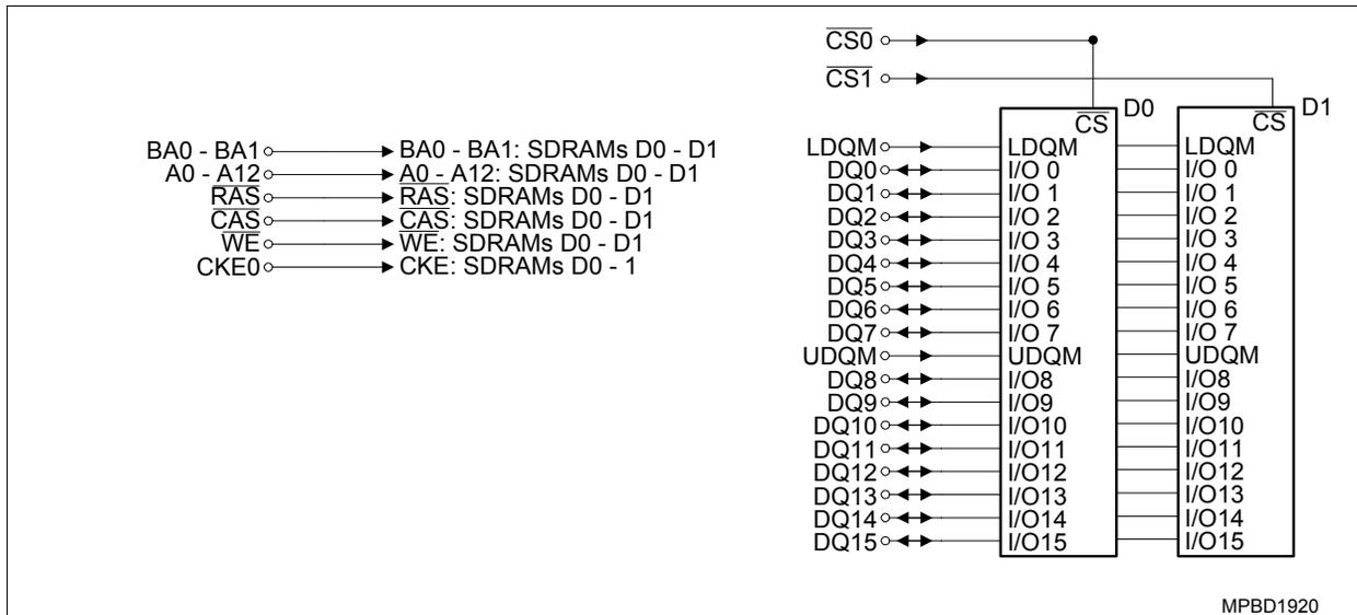
**Figure 2 Block Diagram of Stacked Configuration**
