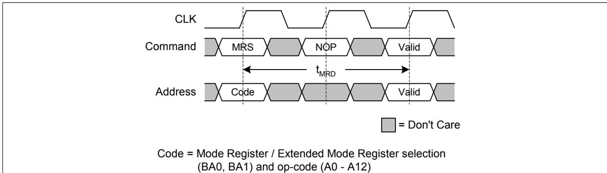
Figure 11 Mode Register Definition
