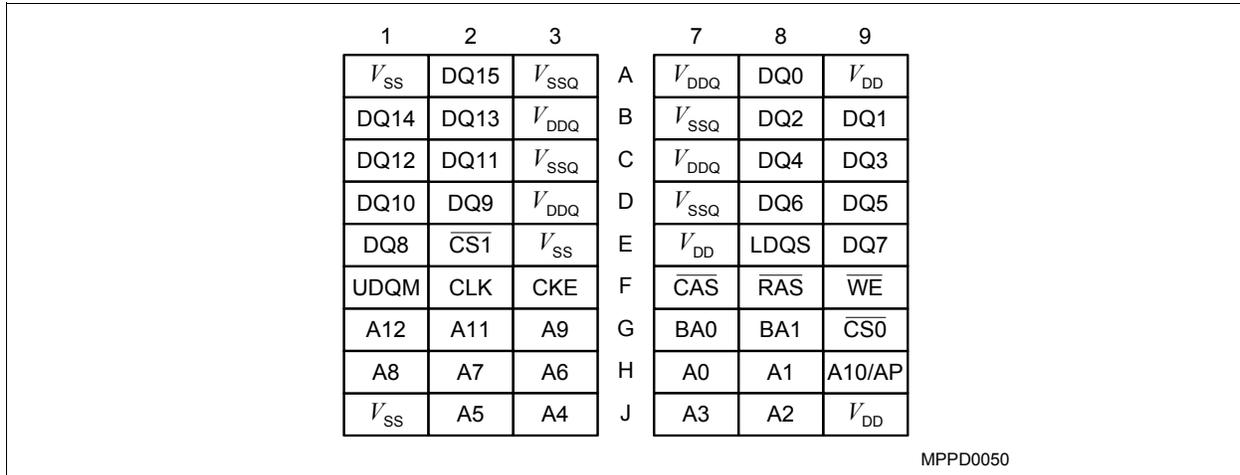
**Figure 1 Standard Ballout 512M Mobile-RAM**
