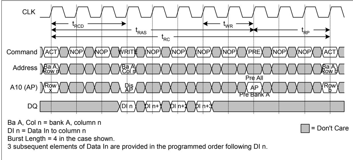
**Figure 29 WRITE Burst (CAS Latency = 3)**
