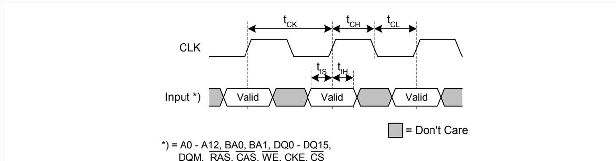
**Figure 8 Address / Command Inputs Timing Parameters**
