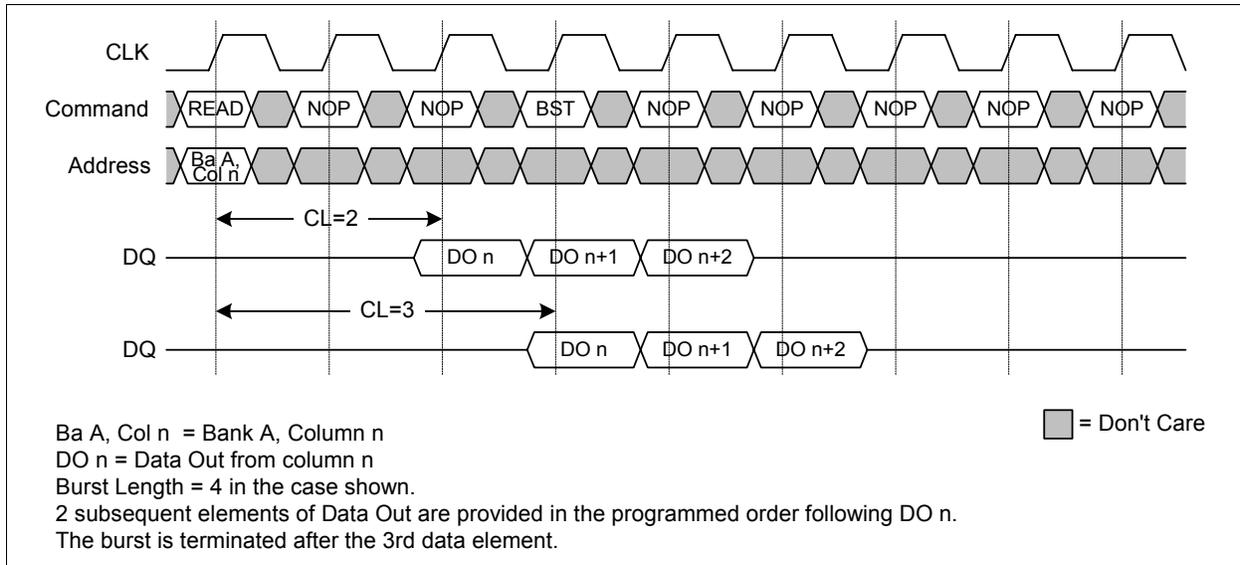
Figure 21 Terminating a READ Burst
