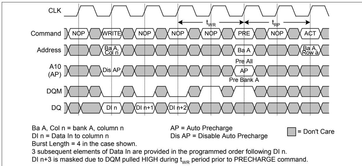
**Figure 37 WRITE to PRECHARGE Timing**
