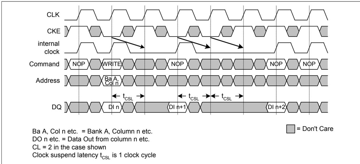
Figure 34 Clock Suspend Mode for WRITE Bursts
