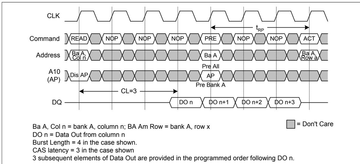
Figure 25 READ to PRECHARGE Timing
