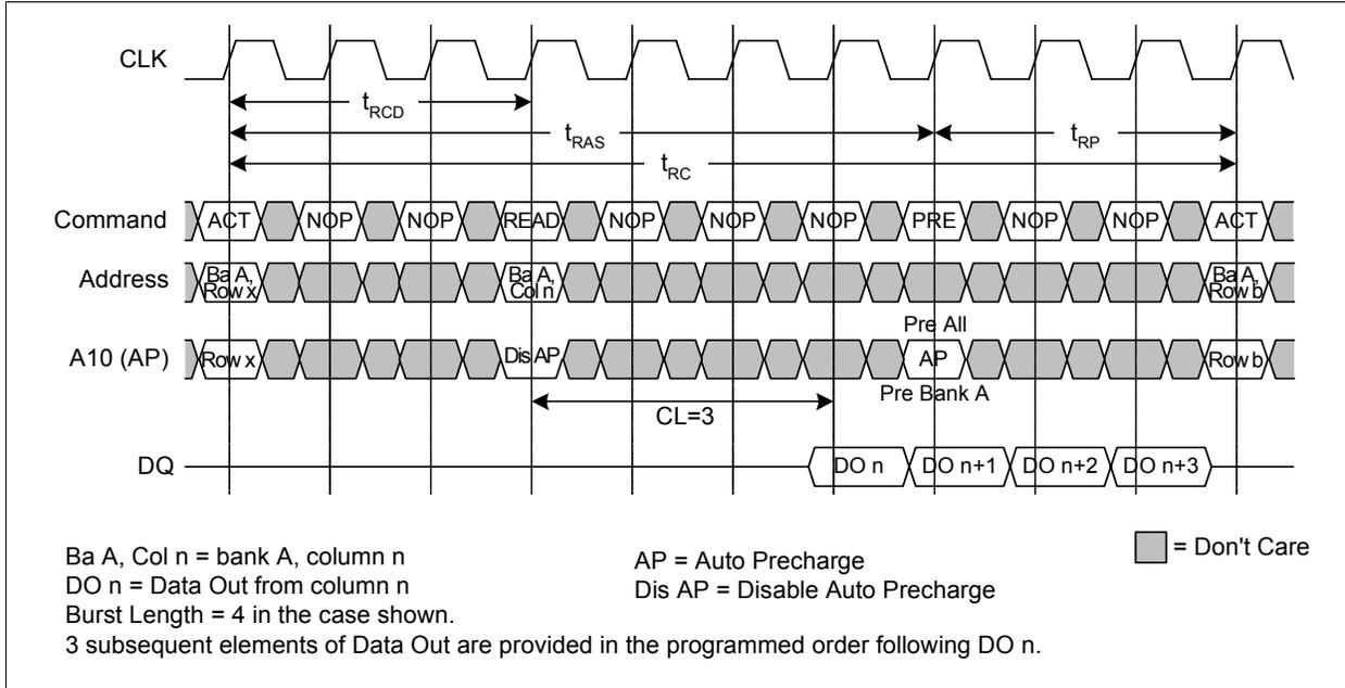
**Figure 17 Single READ Burst (CAS Latency = 3)**
