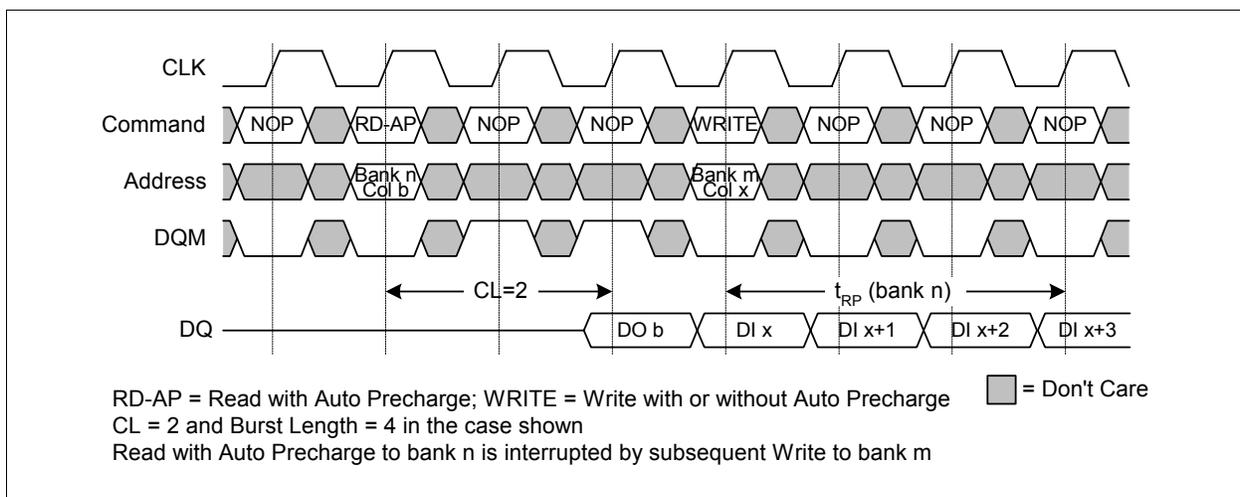
**Figure 41 READ with Auto Precharge Interrupted by WRITE**
