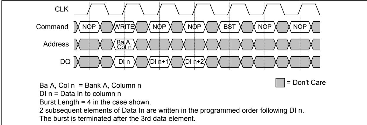
Figure 33 Terminating a WRITE Burs
