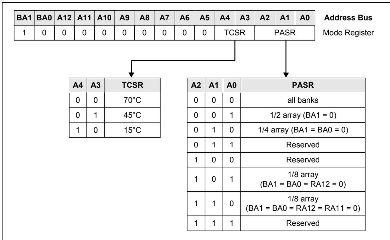
**Figure 6 Extended Mode Register Definition**
