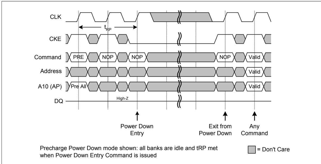
Figure 49 POWER DOWN Entry and Exit
