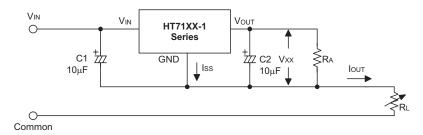
$$I_{OUT} = \frac{V_{XX}}{R_{\Delta}} + I_{SS}$$
