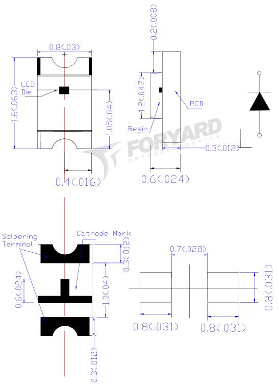
1. Dimension in millimeter [inch], tolerance is  $\pm 0.25$  [.010].
