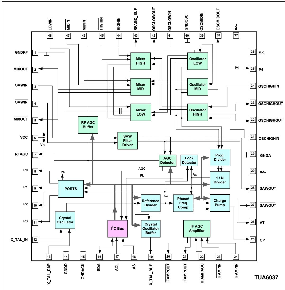
**Figure 6 Functional Block Diagram of TUA 6037**
