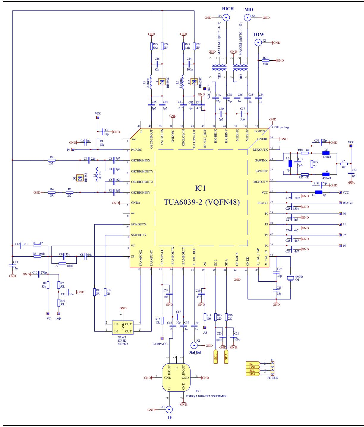
**Figure 9 Circuit diagram for hybrid application (DVB-T / PAL)**
