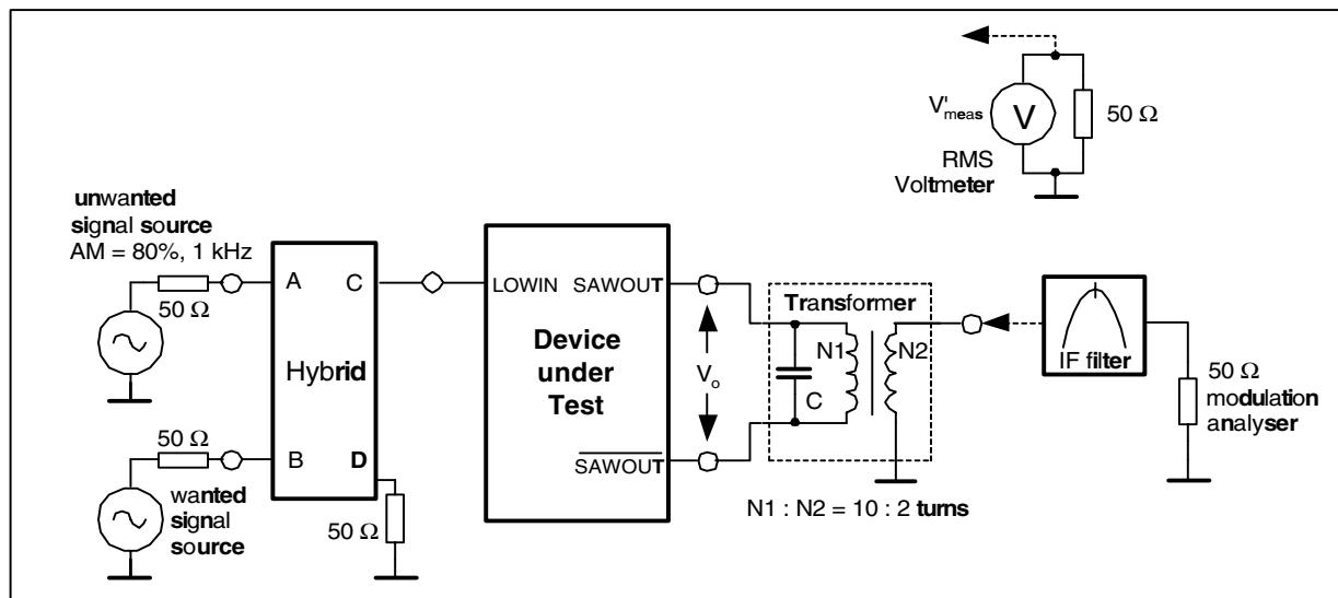
**Figure 19** Cross modulation measurement in LOW band
