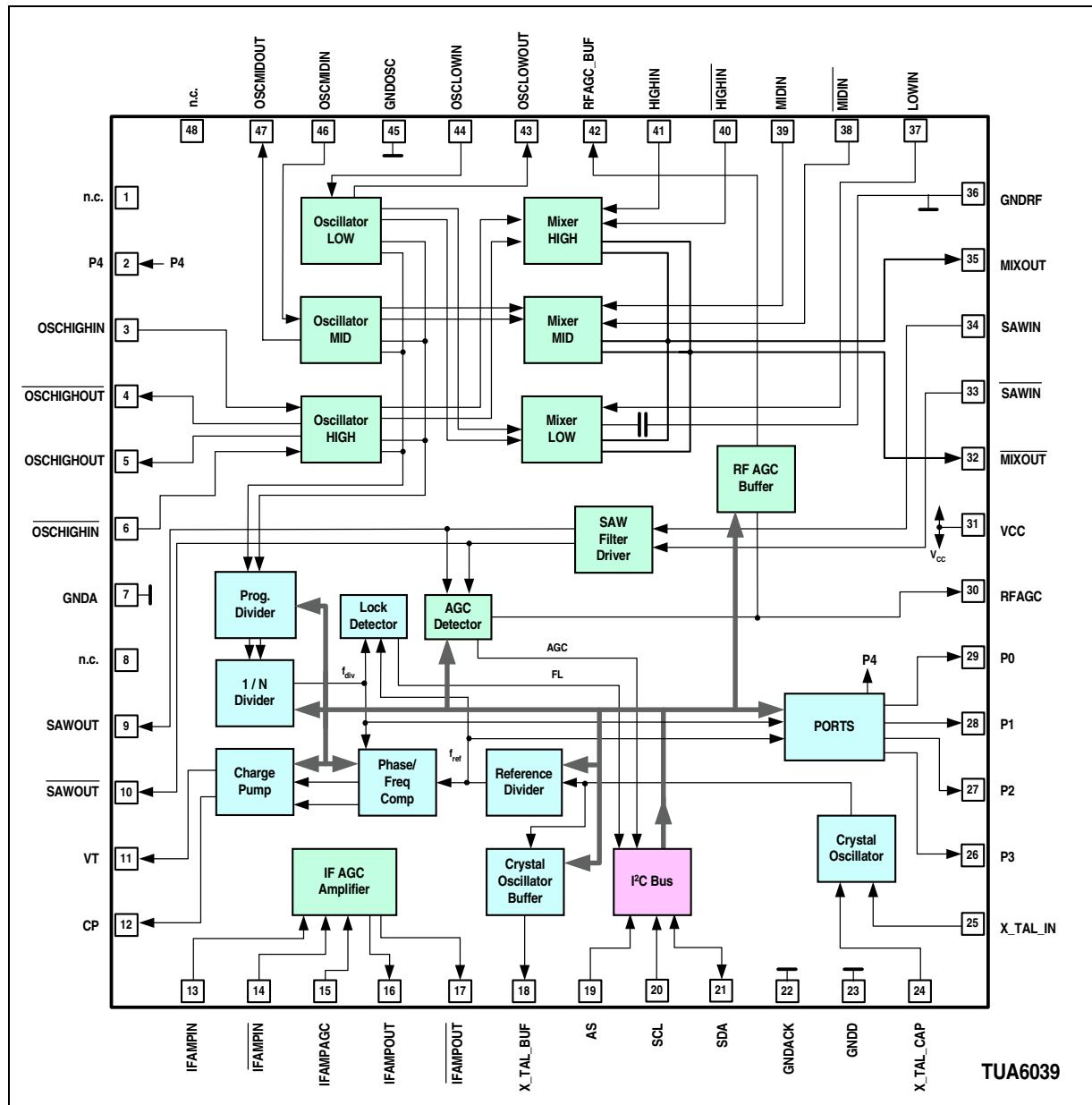
**Figure 5 Functional Block Diagram of TUA 6039**
