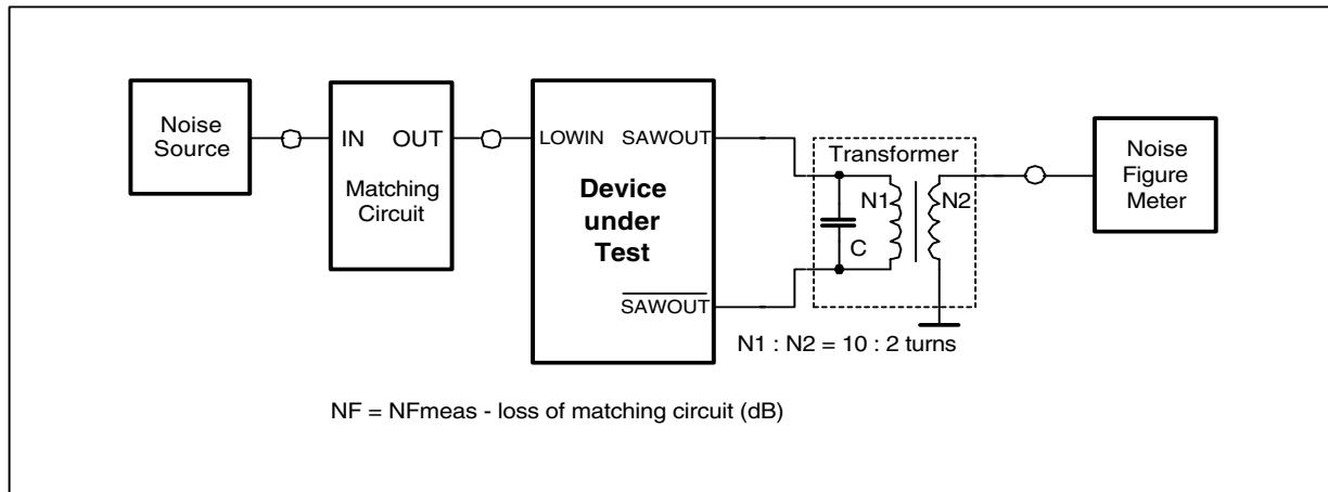
**Figure 17** Noise figure (NF) measurement in LOW band
