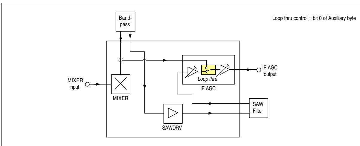
**Figure 7      Functional Block Diagram of Loop thru**
