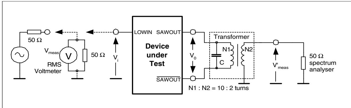
**Figure 14** Gain ( $G_V$ ) measurement in LOW band
