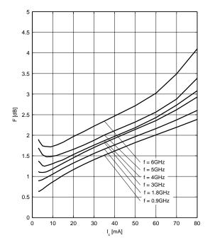
Noise figure F = f(f) $V_{CE} = 3 V, Z_S = Z_{Sopt}$
