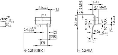
1) Lead width can be 0.6 max. in dambar area
