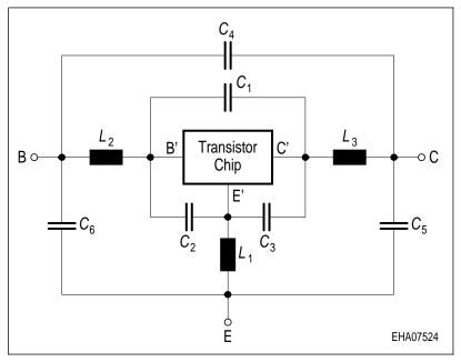
0.85 nΗ  $L_{\mathsf{BO}} =$ 0.51 nΗ 0.69 nΗ  $L_{EO} =$ 0.61 nΗ 0 nΗ L<sub>CO</sub> = 0.49 nΗ C<sub>BE</sub> = 73 fF C<sub>CB</sub>= 84 fF 165  $C_{CE} =$ fF Valid up to 6GHz
