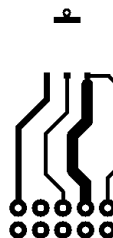
b) 118\text{ }^\circ\text{C/W} when mounted on a minimum pad of 2 oz copper
