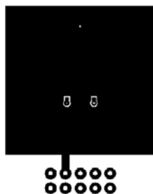
a) 55\text{ }^\circ\text{C/W} when mounted on a 1\text{ in}^2 pad of 2 oz copper
