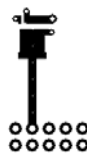
b) 125\text{ }^\circ\text{C/W} when mounted on a minimum pad of 2 oz copper.
