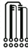
b. 175\text{ }^\circ\text{C/W} when mounted on a minimum pad of 2 oz copper
