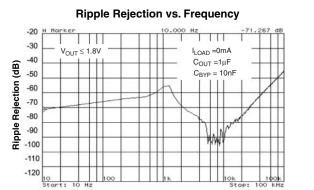
Ripple Rejection vs. Frequency
