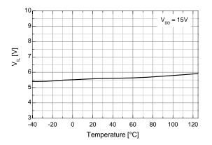
Figure 24. Logic High Input Voltage vs. Temperature
