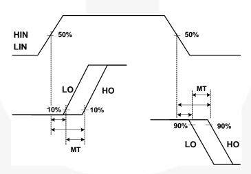
Figure 33. Delay Matching Waveform Definitions
