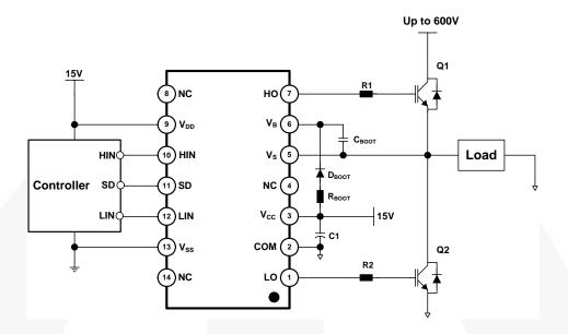
Figure 1. Typical Application Circuit (Referenced 14-DIP)
