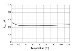
Figure 16. Operating V<sub>CC</sub> Supply Current vs. Temperature
