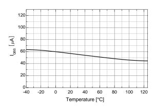
Figure 14. Quiescent V<sub>CC</sub> Supply Current vs. Temperature
