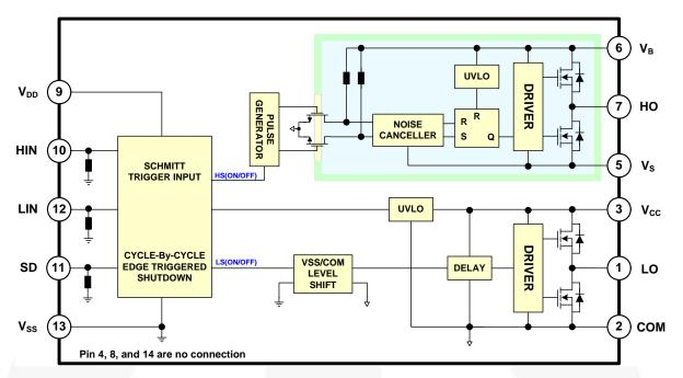
Figure 3. Functional Block Diagram (Referenced 14-Pin)
