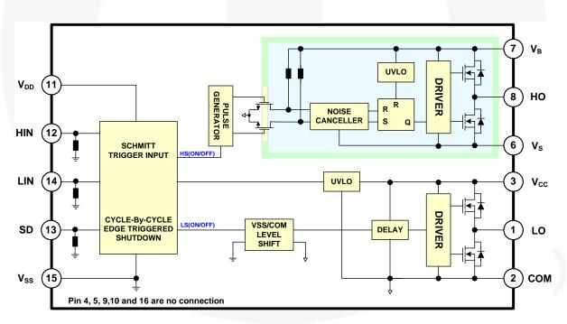
Figure 4. Functional Block Diagram (Referenced 16-SOP)
