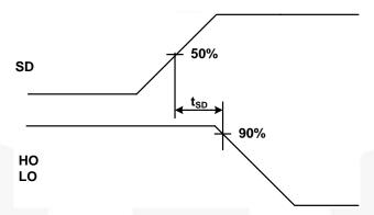
Figure 32. Shutdown Waveform Definition
