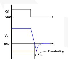
Figure 35. V<sub>S</sub> Waveforms During Q1 Turn-Off
