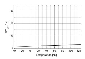
Figure 10. Turn-On Delay Matching vs. Temperature
