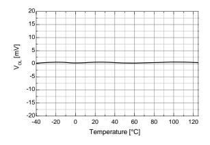
Figure 22. High-Level Output Voltage vs. Temperature
