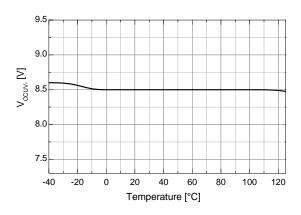
Figure 18. V<sub>CC</sub> UVLO+ vs. Temperature
