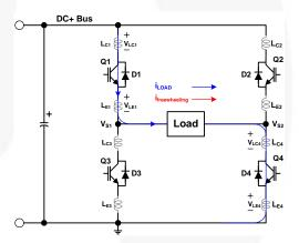
Figure 36. Q1 and Q4 Turn-On
