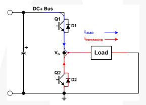
Figure 34. Half-Bridge Application Circuits
