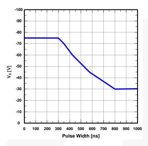
Figure 38. Negative V<sub>S</sub> Transient Chracteristic
