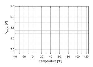
Figure 20. V<sub>BS</sub> UVLO+ vs. Temperature
