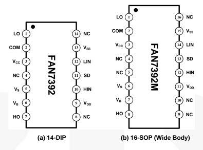
Figure 5. Pin Configurations (Top View)
