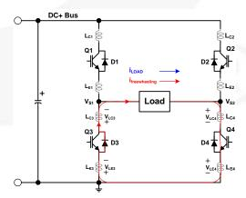
Figure 37. Q1 Turn-Off and D3 Conducting
