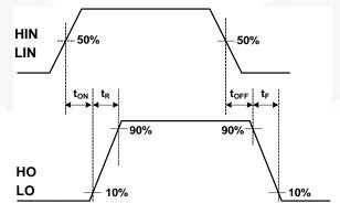
Figure 31. Switching Time Waveform Definitions
