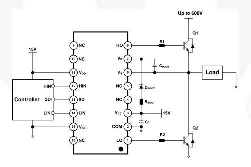
Figure 2. Typical Application Circuit (Referenced 16-SOP)
