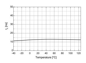
Figure 8. Turn-On Rise Time vs. Temperature
