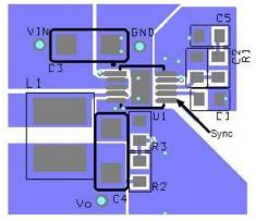
Figure 16. Recommended PCB Layout
