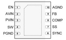
Figure 2. Pin Configuration (Top View)
