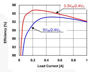
Figure 11. Efficiency vs. Load Current
