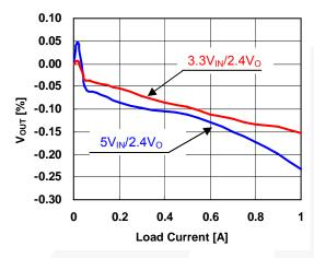
Figure 10. Normalized Vout vs. Load Current
