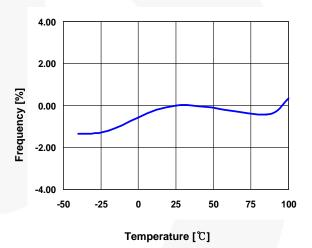
Figure 13. Normalized Oscillation Frequency vs.
