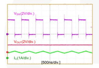
Figure 6. PWM Operation with 1A Load
