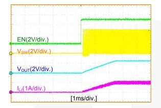
Figure 4. EN Startup with 1A Load
