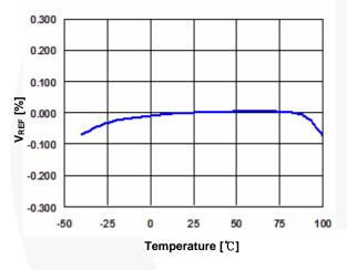
Figure 12. Normalized V<sub>REF</sub> vs. Temperature
