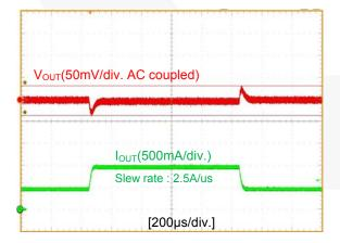
Figure 8. Load Transient Response(Step-up/down)
