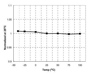
Figure 7. High-Side V<sub>cc</sub> (HV<sub>cc</sub>) Stop vs. Temperature
