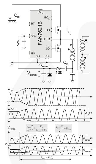
Figure 27. Current Sensing Using Resonant Capacitor Voltage
