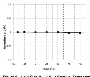
Figure 8. Low-Side  $V_{cc}$  (LV<sub>cc</sub>) Start vs. Temperature
