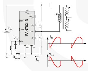
Figure 25. Half-Wave Sensing
