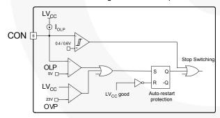
Figure 21. Internal Block of Control Pin
