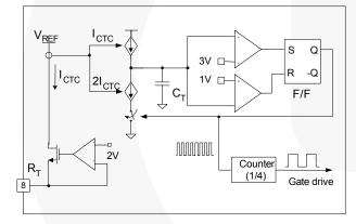
Figure 17. Current Controlled Oscillator
