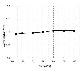
Figure 11. OLP Protection Voltage vs. Temperature
