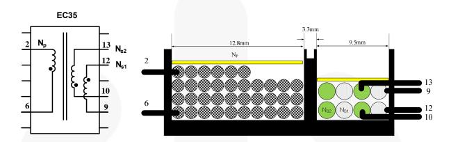
Figure 30. Transformer Construction
