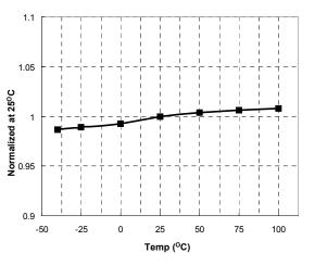
Figure 13.  $R_T$  Voltage vs. Temperature
