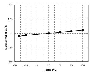
Figure 12. LV<sub>CC</sub> OVP Voltage vs. Temperature
