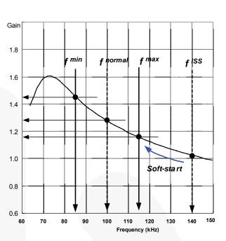
Figure 18. Resonant Converter Typical Gain Curve
