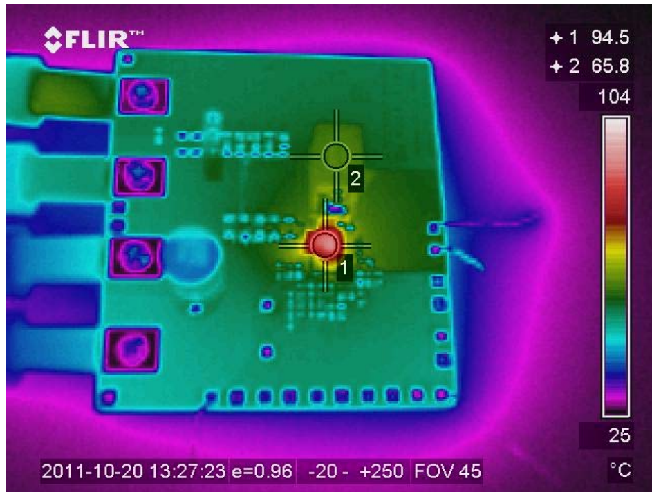
Figure 45: Thermal Image of the Board at 16A Load, Test Point 1 is IR3895, Test Point 2 is inductor
