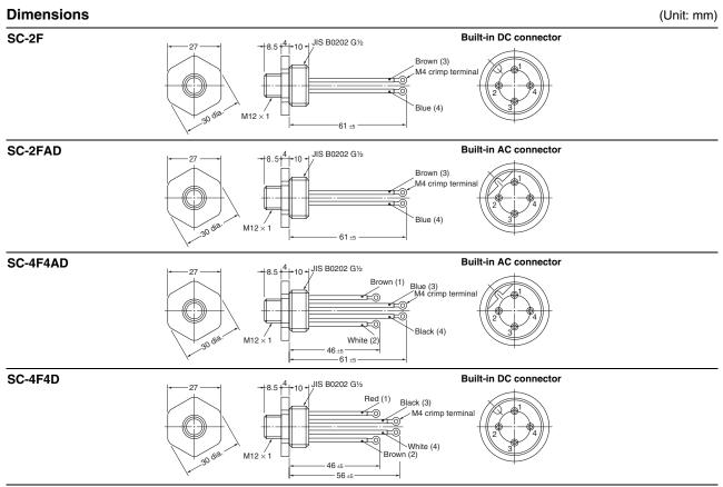
Note: 1. Each dimension has a tolerance of  $\pm 0.4$  mm unless otherwise specified.
