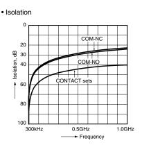
1-(2). High frequency characteristics (Impedance  $75\Omega$ )
