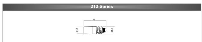
Dimensions in mm (Typical) Not to scale Green dot on base indicates centre contact cathode -ve. Colour dot on product denotes LED colour.
