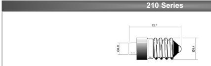
Dimensions in mm (Typical) Not to scale Centre contact Anode +ve as standard Colour dot on product denotes LED colour.
