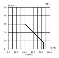
^ = Products must be derated according to the derating
