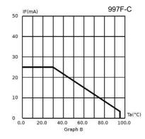
^ = Products must be derated according to the derating information. Each derating graph refers to specific LEDs.
