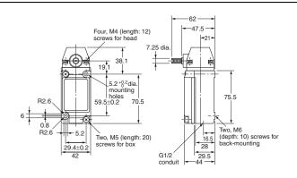
Note: Unless otherwise specified, a tolerance of  $\pm 0.4$  mm applies to all dimensions.
