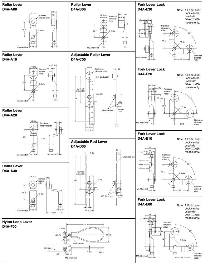
Note: Unless otherwise specified, a tolerance of  $\pm 0.4$  mm applies to all dimensions.
