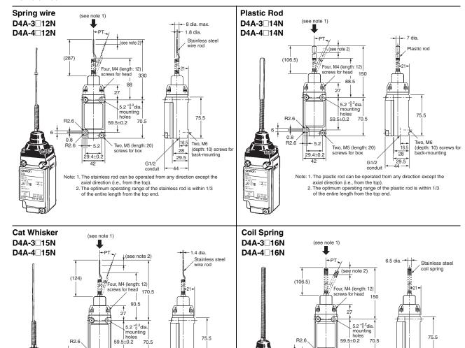
Note: Unless otherwise specified, a tolerance of  $\pm 0.4$  mm applies to all dimensions.
