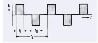
2. Periodic recurrence of two unequal energizing pulses
