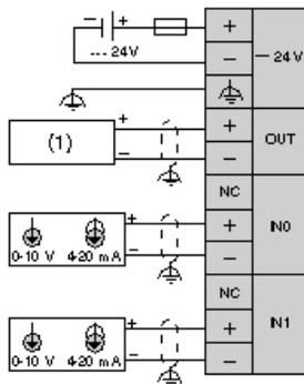
(1) Voltage/current preactuator
